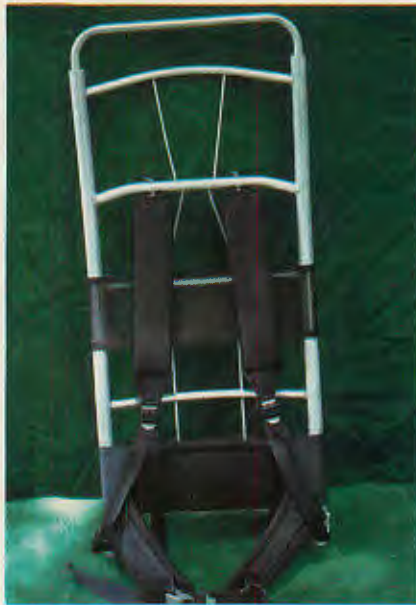
Kelty® frame and padded hip belt with nylon-mesh back bands. Frame is excellent example of H-design. All joints are welded for strength.
